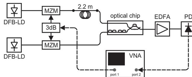
Fig. 6. Schematic of the 2-tap microwave photonic filter.
