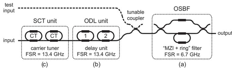
Fig. 2. Schematic of the delay structure employed to demonstrate the single-chip SCT-based optical delay line: (a) optical sideband filter (OSBF); (b) optical delay line (ODL) unit; (c) separate carrier tuning (SCT) unit.
