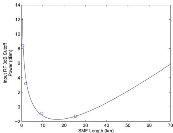
Fig. 9. Measured (circle) and simulated (line) input RF power at which the Brillouin gain drops by 3 dB below its maximum value of 30 dB, for different Brillouin medium lengths.
