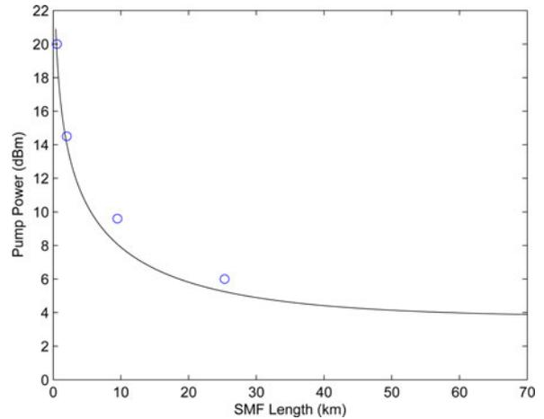
Fig. 8. Measured (circle) and simulated (line) pump power required to achieve 30 dB rejection level for different Brillouin medium lengths.
