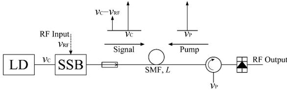
Fig. 1. Fundamental structure of SBS-based microwave photonic filter.
