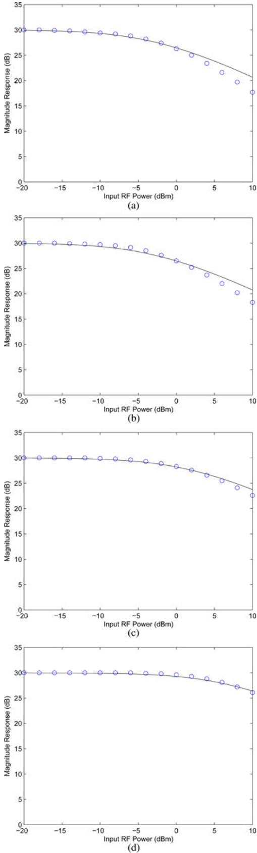
Fig. 6. Measured (circle) and simulated (line) filter rejection level for different input RF powers. SMF length: (a) 25.32 km, (b) 9.49 km, (c) 2.01 km, and (d) 0.57 km.
