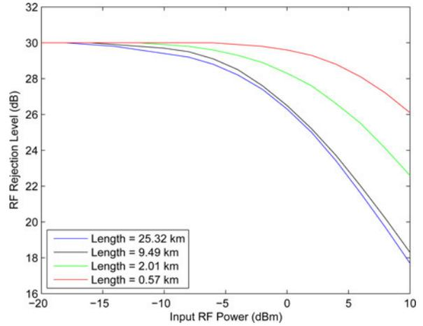
Fig. 7. Experimental filter rejection level for different Brillouin medium lengths.
