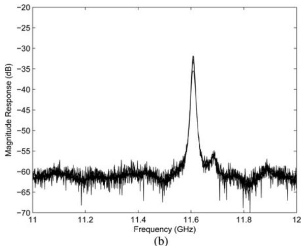
Fig. 4. Frequency response for input RF powers equal to  $-20$  dBm,  $-15$  dBm, ...,  $10$  dBm. SMF length: (a)  $25.32$  km and (b)  $0.57$  km.
