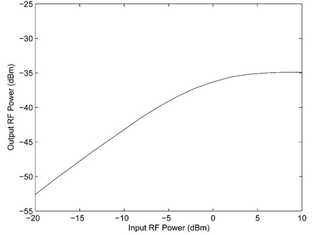
Fig. 2. Measured output RF power as a function of input RF power.
