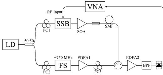
Fig. 3. Experimental setup of the SBS-based microwave photonic filter.
