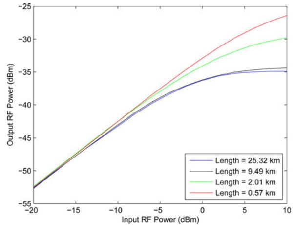
Fig. 5. Experimental input–output RF power relationship for different Brillouin medium lengths.
