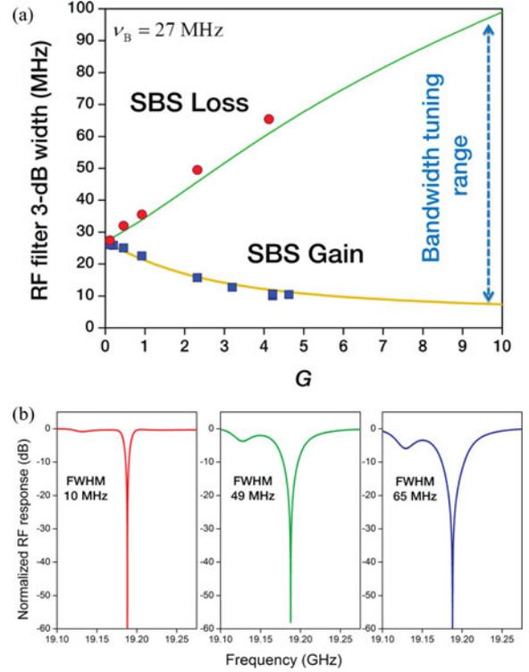
Fig. 3. (a) RF filter 3-dB bandwidth reconfigurability as functions of the SBS gain parameter,  $G$ . Solid lines represent simulation results with SBS linewidth of 27 MHz, while the scatter plots represent experimental data, for SBS filter in 650 m of SMF. In the experiments variation of  $G$  was obtained by changing the pump power. (b) The measured filter responses, showing optimized peak rejection independent of the bandwidth.
