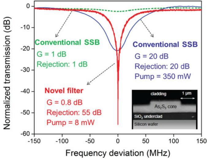
Fig. 2. Experimental result of MWP notch filter response using on-chip SBS with sub-1 dB gain. Blue trace indicates conventional filter using SSB modulation and SBS loss spectrum [14]. Red trace indicates notch response obtained from novel complex sideband processing [7] and SBS gain spectrum. The novel technique leads to an increase in filter resolution (47 MHz full-width at half maximum) and ultra-high enhancement of the peak rejection ( $>55$  dB), achieved with only 8 mW of pump power.
