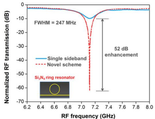
Fig. 4. Experimentally measured MWP notch filter response using a low loss  $\text{Si}_3\text{N}_4$  ring resonator [8]. Implementing the complex sideband processing [6]–[8] led to a peak rejection enhancement of  $>50$  dB relative to conventional SSB scheme.
