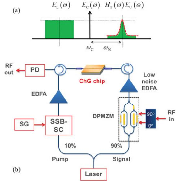
Fig. 1. (a) Illustration of the sideband amplitudes to achieve a necessary cancellation condition in a novel high extinction notch filter. (b) Experimental setup of ultrahigh rejection notch filter using SBS on chip. SG = RF signal generator, PD = photodetector, SSB-SC = single sideband suppressed carrier modulator, DPMZM = dual parallel Mach-Zehnder modulator.
