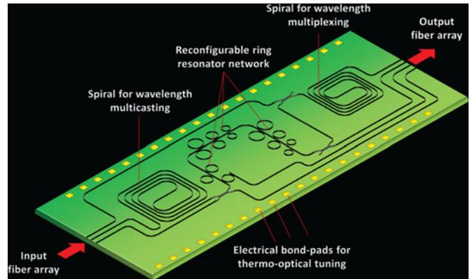
Fig. 5. Illustration of the envisioned general purpose ASP architecture combining ultrafast nonlinear optics for signal copies generation (for example wavelength multicasting via on chip FWM) and reconfigurable linear optical filtering (for example Vernier ring resonators tunable using thermo-optical tuning).
